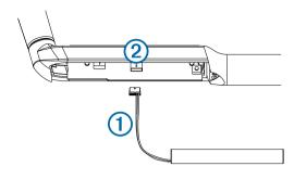
The connector fits into the port only one way. Forcing the connector into the port may damage it.
